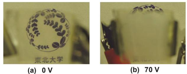
**Fig.8 Voltage drive of junction cell in curved state with a bending radius of 10 mm.**
