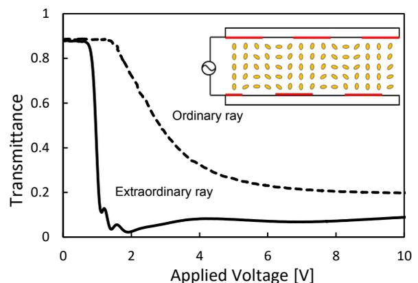
Fig. 5 Electro-optical properties in the LC cell with hole-patterned electrode on both side of the substrates.
