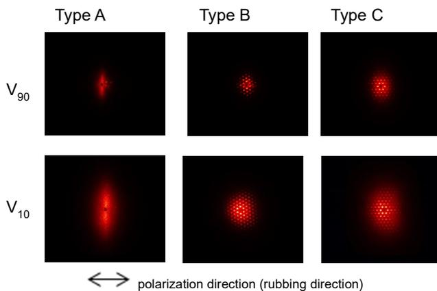
Fig. 3 Light scattering patterns in three cells by applying voltage of  $V_{90}$  and  $V_{10}$ .
