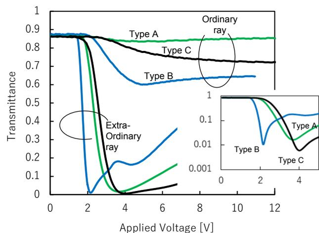
Fig. 2 Electro-optical properties of reverse mode cells.
