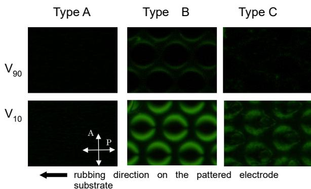
Fig. 4 POM images in three cells by applying voltage of  $V_{90}$  and  $V_{10}$ .
