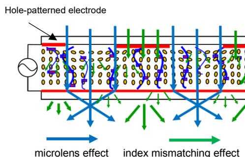
Fig. 1 Schematic model of scattering effect of combined cell.
