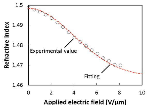
**Fig. 3 Measured refractive index modulation (wavelength: 1,000 nm) of PSBPLCs by the extended Kerr effect. The direction of the measured refractive index is a normal direction of the electric field. The electric field is a square wave (frequency: 1 kHz).**
