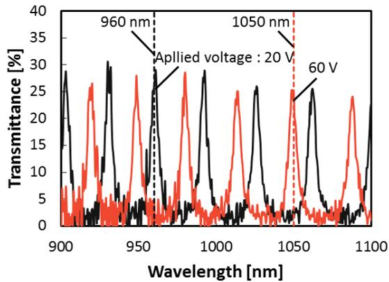
**Fig. 4 Measured transmission spectrum changes of the fabricated PSBPLC etalon filter according to the applied voltage.**
