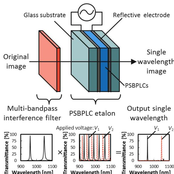
Fig. 1 Structure and transmittance of the electrically tunable filter using the PSBPLC etalon filter.
