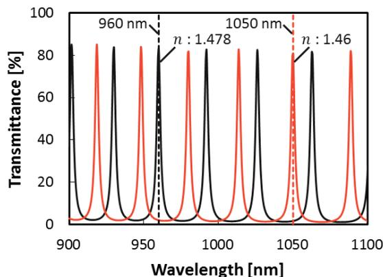
**Fig. 2 Simulated transmission spectrum changes of the PSBPLC etalon filter caused by refractive index modulation**
