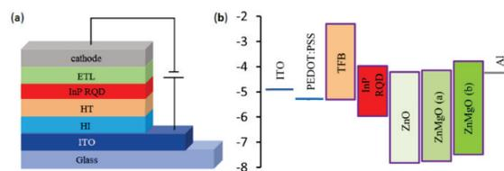
**Fig. 1 a) Basic device structure of InP QLED with ITO anode; b) Energy band diagrams of InP QLEDs with ZnO, Zn<sub>0.95</sub>Mg<sub>0.05</sub>O (a), and Zn<sub>0.85</sub>Mg<sub>0.15</sub>O (b) ETLs**
