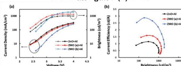
**Fig. 2 Current efficiency of the InP R-QLED devices utilizing ZnO, Zn<sub>0.95</sub>Mg<sub>0.05</sub>O, and Zn<sub>0.85</sub>Mg<sub>0.15</sub>O ETLs**
