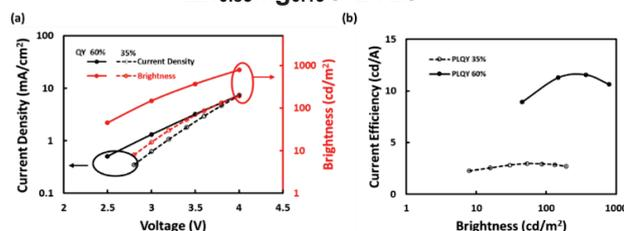
**Fig. 3 Characteristics of QLED devices, utilizing InP-based RQDs with 35% and 60% PLQY: (a) Current density and brightness; (b) Current efficiency.**
