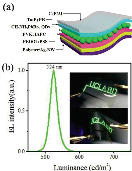
**Fig. 3** (a) The device structure of flexible CH<sub>3</sub>NH<sub>3</sub>PbBr<sub>3</sub> QDs based LEDs; (b) EL spectra and images of the flexible CH<sub>3</sub>NH<sub>3</sub>PbBr<sub>3</sub> QDs based LEDs and devices tailored with abbreviations of UCLA & BIT shown in the inset.
