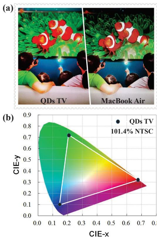
**Fig. 5** (a) A comparison between CH<sub>3</sub>NH<sub>3</sub>PbBr<sub>3</sub> QDs enhanced LCD screen (left) and MacBook LCD screen (right) (Image source from 3M website); (b) Color gamut triangle of CH<sub>3</sub>NH<sub>3</sub>PbBr<sub>3</sub> QDs enhanced LCD screen in CIE 1931 diagram.
