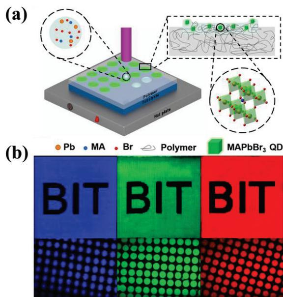
**Fig. 4** (a) Schematic diagram of the in situ inkjet printing strategy. (b) The optical images and microscopic fluorescent images of printed PQDs patterns with red, green and blue colors under UV light illuminations
