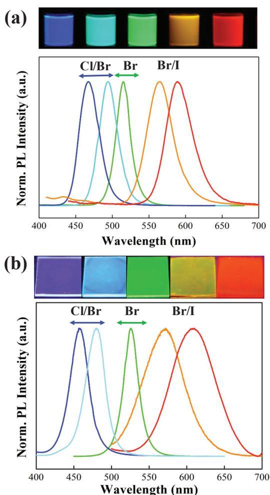
**Fig. 1** (a) Optical images and emission spectra of  $\text{CH}_3\text{NH}_3\text{PbX}_3$  QDs and (b)  $\text{CH}_3\text{NH}_3\text{PbX}_3/\text{PVDF}$  composite films under a 365 nm UV lamp.
