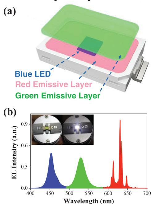
**Fig. 2** (a) The device structure of  $\text{CH}_3\text{NH}_3\text{PbBr}_3/\text{PVDF}$  composite film based SMD LEDs; (b) EL spectra and photographs (shown in the inset) of as-fabricated SMD white LEDs.
