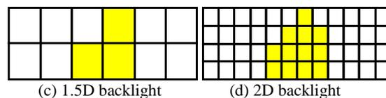
Figure (2) Local dimming technology
