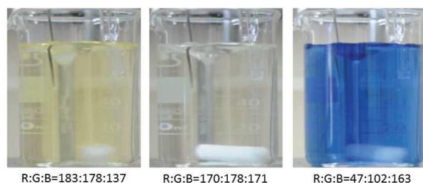
Fig. 1 Colors for B-R reaction<sup>5)</sup>
