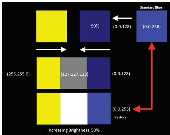
Fig. 2 Color mixing for the standard color display
