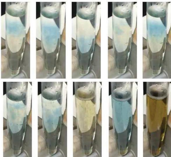
Fig. 4 Color variations and frequency can be controlled by pH and temperature of the compositions
