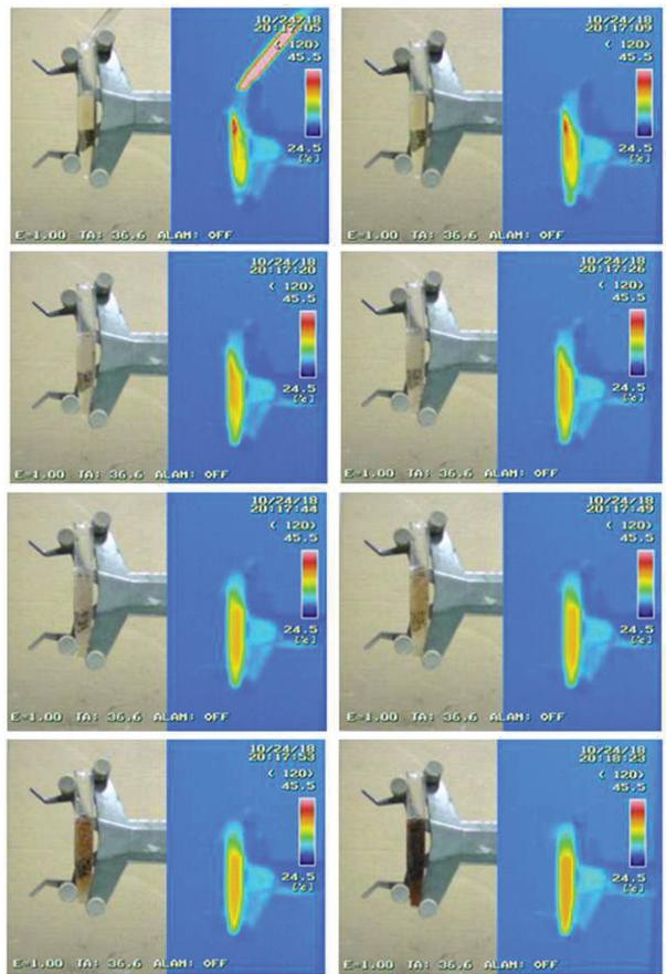
Fig.5 Temperature distribution of mixing chemicals
