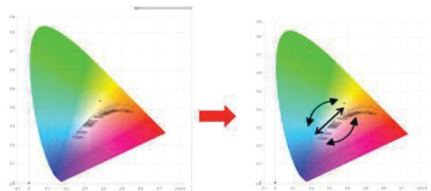
Fig. 6 Dynamic variations on the display color coordinate as function of pH and temperature
