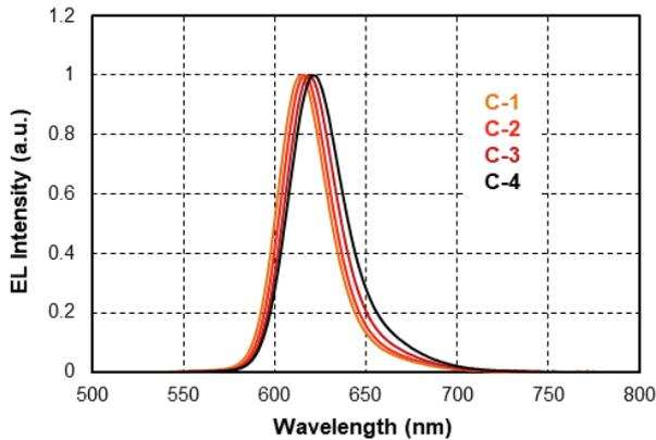
Fig. 1 Normalized TE spectra of Device C at a current density of 10 mA/cm<sup>2</sup>.
