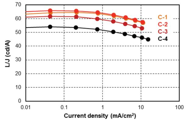
Fig. 3 Current density vs. L/J curves in Device C.
