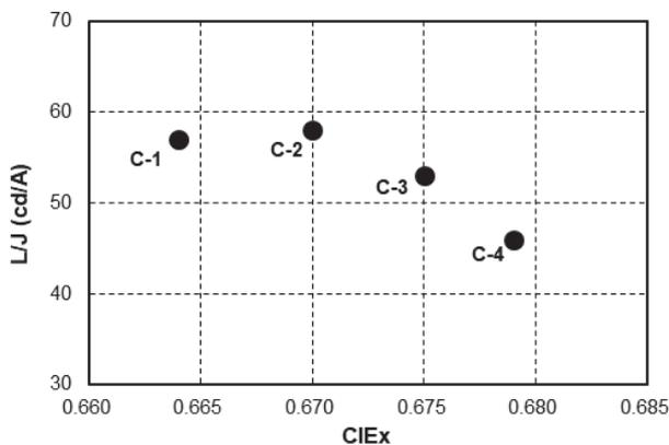
Fig. 2 CIEx coordinate vs. L/J in Device C at a current density of 10 mA/cm<sup>2</sup>.
