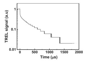
Figure 1. TrEL signal of pristine OLED with pure CbzBzCN in emitting layer.
