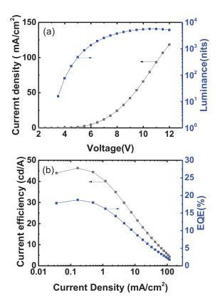
Figure 2. (a) current density and luminance versus voltage, (b) current efficient and external quantum efficiency versus current density of OLED with FIrpic emitter.
