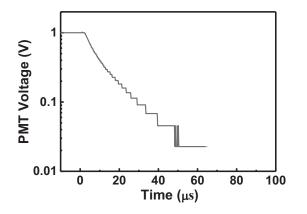
Figure 3. TrEL signal of OLED with FIrpic emitter and CbzBzCN host in emitting layer.
