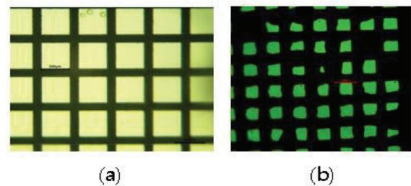
**Fig. 4. (a) Optical image of cathode; (b) Optical image of electroluminescence.**
