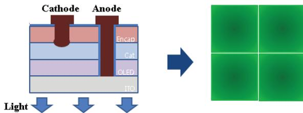
**Fig.6. Concept of OLED tile device.**
