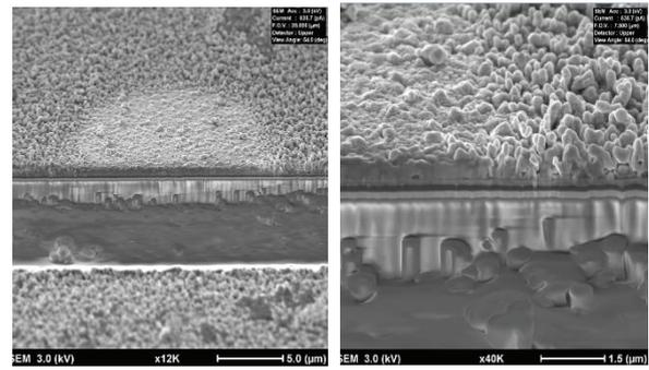
**Fig.3. Cross-section images of micropixel and hole.**
