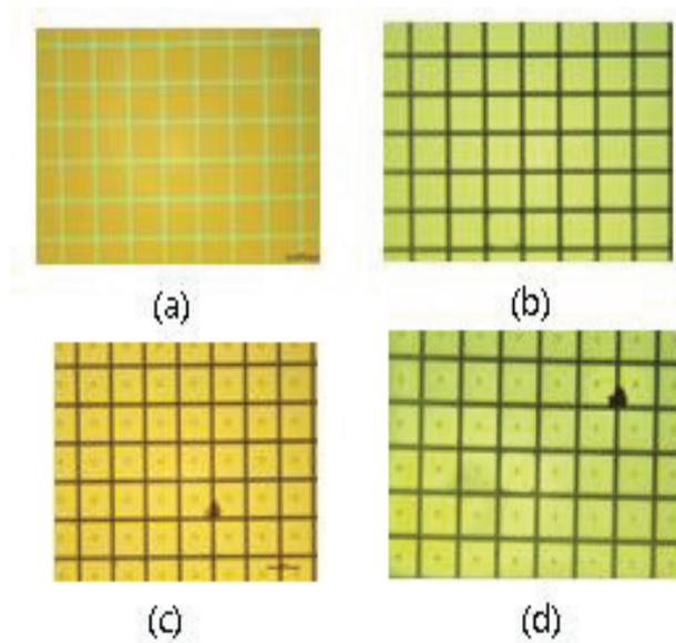
**Fig. 2. Optical images of OLED micropatterning pixels. (a) PR patterning by photolithography; (b) Etching of encapsulation, cathode, OLED layers; (c) Hole patterned by photolithography; (d) Hole etching.**
