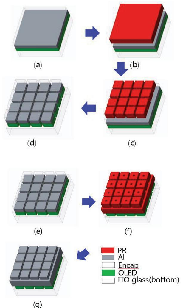
Fig. 1. Schematic fabrication process of OLED micropatterning pixels. (a) OLED, cathode deposition and encapsulation; (b) PR coating; (c) PR patterning by photolithography; (d) Etching of encapsulation, cathode, OLED layers; (e) Sidewall insulation by plasma polymer; (f) Hole patterned by photolithography; (g) Etching and second cathode deposition.
