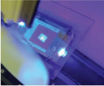
**Fig.5. Photoluminescence image of micropatterned blue fluorescence OLED.**
