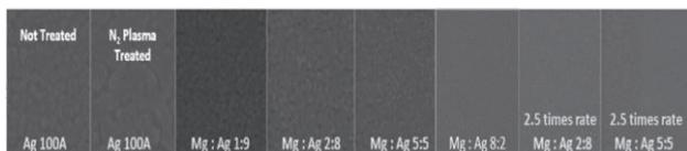
**Fig. 3 Surface status of Mg:Ag based on deposition conditions measured by SEM**
