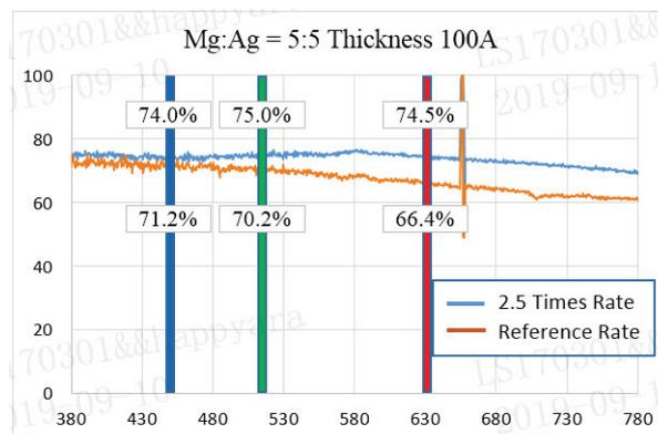
**Fig. 4 Transmittance based on deposition rate**
