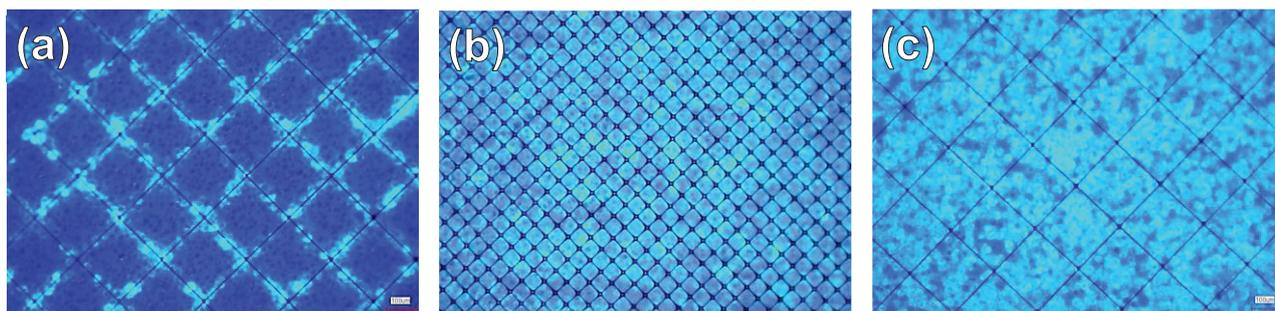
**Fig. 4** Microscope images of light emitting from the PELDs on the Ag-grid electrodes (a), (b) without and (c) laminated with PEDOT:PSS. Spacing between the lines: (a) 200  $\mu\text{m}$ , (b) 50  $\mu\text{m}$ , and (c) 200  $\mu\text{m}$ .
