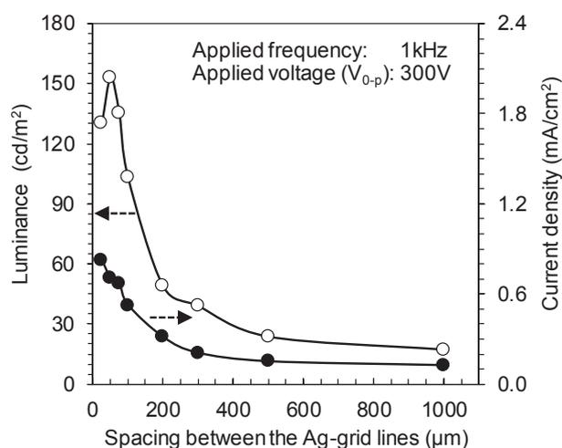
**Fig. 2** Current and luminance versus spacing between the Ag-grid lines of the Ag-grid electrodes without PEDOT:PSS of the developed PELD.
