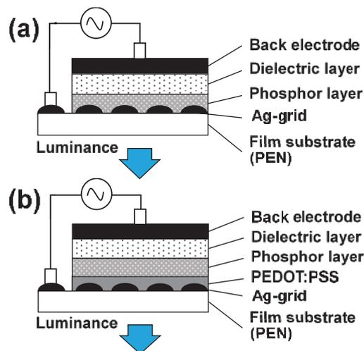
**Fig. 1** Structure of the PELDs on the Ag-grid electrodes (a) without and (b) laminated with PEDOT:PSS.
