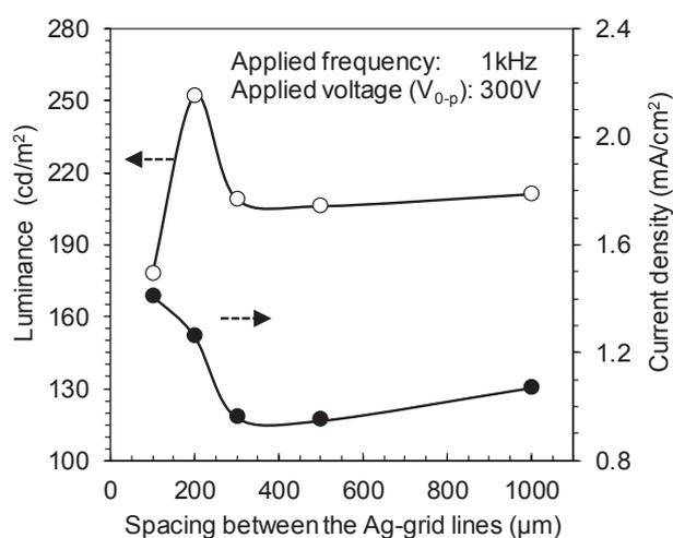
**Fig. 3** Current and luminance versus spacing between the Ag-grid lines of the Ag-grid electrodes laminated with PEDOT:PSS of the developed PELDs.
