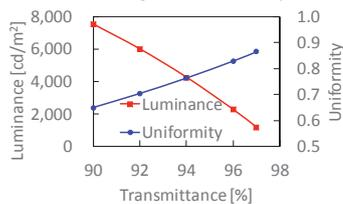
**Fig. 3 Dependence of luminance on transmittance**
