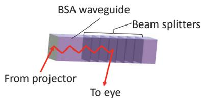
**Fig. 2 Beam splitter array waveguide**
