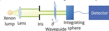
**Fig. 4 Measurement setup of transmittance**
