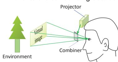
**Fig. 1 See-through head mounted display**
