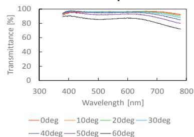
**Fig. 5 Measurement result of transmittance**
