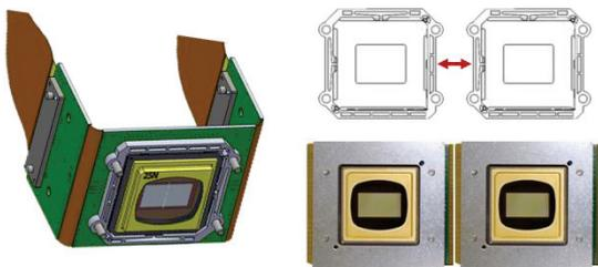
Fig. 6 V-Module design for multiple head exposure with minimal lateral distance
