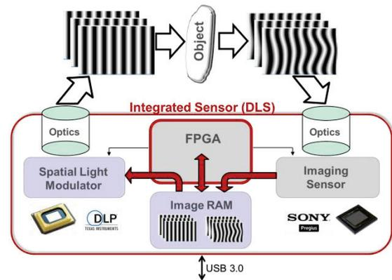
Fig. 4 Architecture of 3D measurement system [8]
