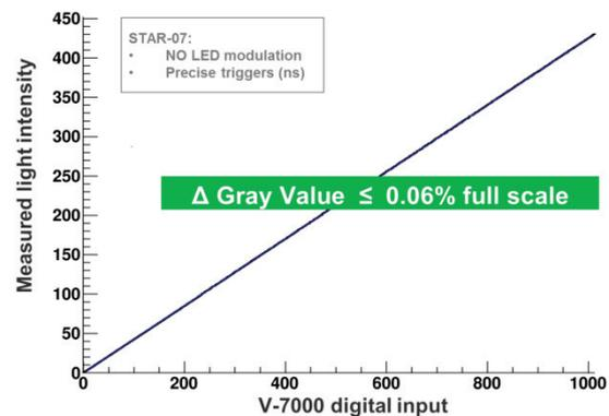
Fig. 5 Linearity of V-Module generated grayscale
