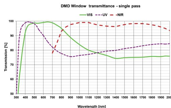
Fig. 1 DMD window transmittance
