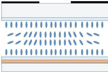
Fig. 4 Design of the UV<sup>2</sup>A negative LC lens
