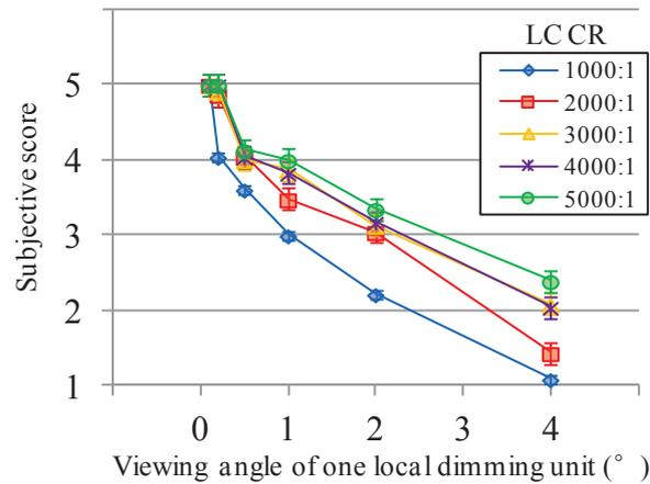
**Fig. 5** Experimental results, with mean scores and standard deviations for each viewing angle of one local dimming unit under each contrast ratio of the liquid crystal panel.
