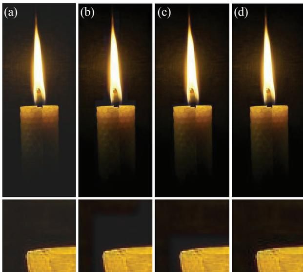
**Fig. 2** Simulation of the perceptual results. (a) Low dynamic range image on the normal LCD without mini-LED backlight; (b) HDR image on the LCD with a mini-LED backlight, local dimming unit size  $10\times 10$  mini-LEDs; (c) HDR image on the LCD with a mini-LED backlight, local dimming unit size  $5\times 5$  mini-LEDs; (d) HDR image on the LCD with a mini-LED backlight, local dimming unit size  $1\times 1$  mini-LED.
