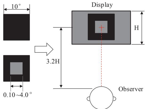
**Fig. 3** Experimental settings, with at the left the background outer square (top) and the leakage inner square (bottom). The picture on the right hand side shows the appearance of the stimulus on the display. The distance between the observer and the display was  $3.2H$  ( $3.2$  times the display height).
