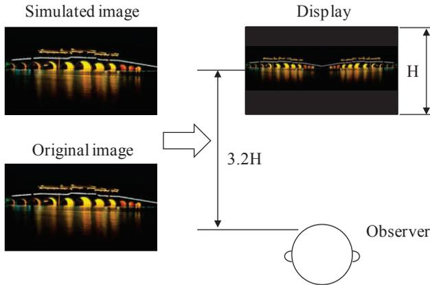
**Fig. 4** Experimental settings, with at the left the simulated image (top) and the original image (bottom). The images were displayed side by side with random order. The image presenting on the right side is left and right reversed.
