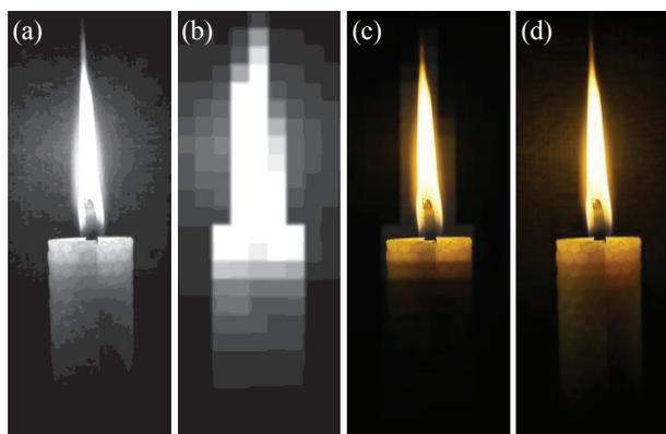
**Fig. 1** The image rendering procedure of the high dynamic range LCD with a mini-LED backlight. (a) The maximum light image with each pixel the maximum value of RGB channels; (b) mini-LED lighting image according to the maximum light image and the local dimming unit allocation strategy; (c) mini-LED backlight through the original LC panel modulation; (d) mini-LED backlight through pixel compensated LC panel.
