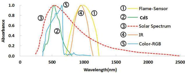
Fig. 2 Comparison of spectrum of CdS to various photo-electronics devices
