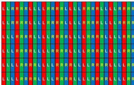
**Fig. 2 Interleaved left-eye and right-eye images**
