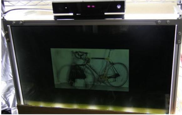
**Fig. 4** 4K Autostereoscopic display used in the experiment.
