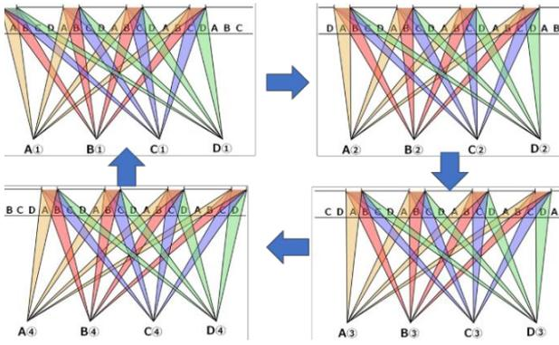
**Fig. 1 Time-division quadruplexing parallax barrier. (Blue arrows indicate the order of time sequence.)**
