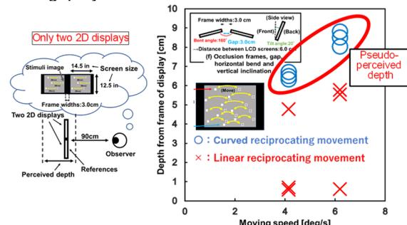
Fig. 10 Pseudo-perceived depth by using fame, gap and curved reciprocating movement
