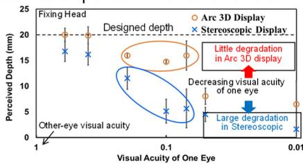
Fig. 5 Little depth degradation in Arc 3D display by decreasing one-eye visual acuity
