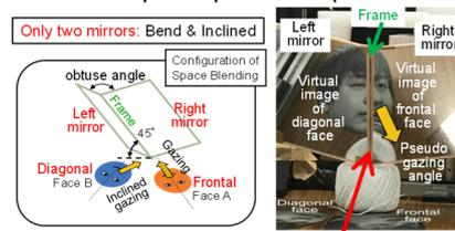
Fig. 11 Configuration of Space blending of two face orientations using two mirrors
