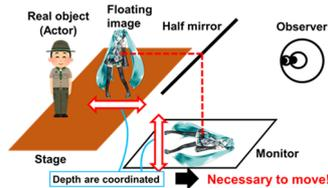
Fig. 8 Problem in floating 3D image using a half mirror
