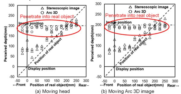
Fig. 7 Arc 3D image penetration into real object by moving (a) head and/or (b) Arc 3D image
