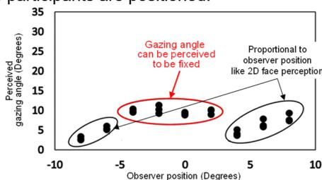
Fig. 13 Perceived gazing direction dependence on observer position by space blending of two face orientations
