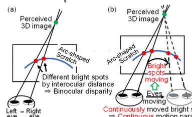
Fig. 3 Principle of Arc 3D display: an arc-shaped scratch corresponds to a pixel of usual display
