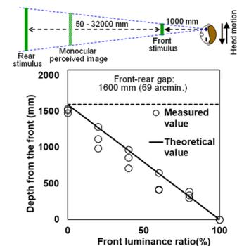
Fig. 2 Continuous motion parallax in DFD display
