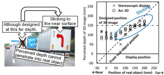
Fig. 6 Floating image sticking to real object surface
