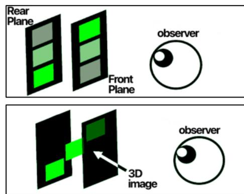
Fig. 1 Principle diagram of DFD display
