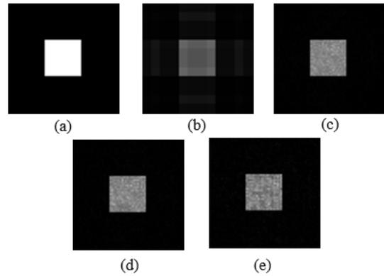
Fig. 3 (a)The input image; (b) the image after grating; (c) the image after the continuous phase DOE; (d) the image after the 16-level phase DOE; (e) the image after the 8-level phase DOE.
