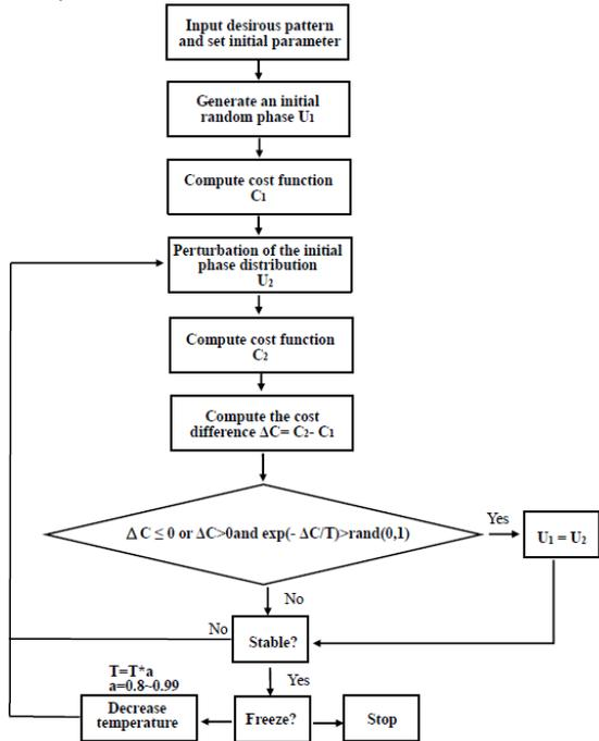
Fig. 2 A flow chart of the simulated annealing algorithm.
