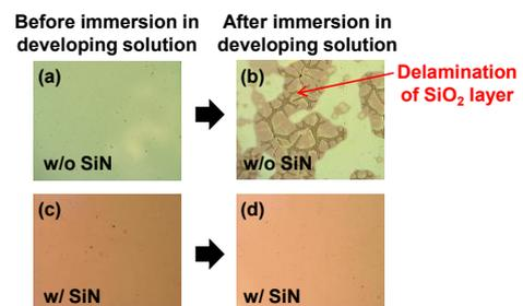
Fig. 2. Optical micrographs of PI films (a), (c) before and (b), (d) after immersion in developing solution. Note that a 200-nm-thick  $\text{SiO}_2$  layer was sputtered onto the PI films with and without a 50-nm-thick SiN underlayer.
