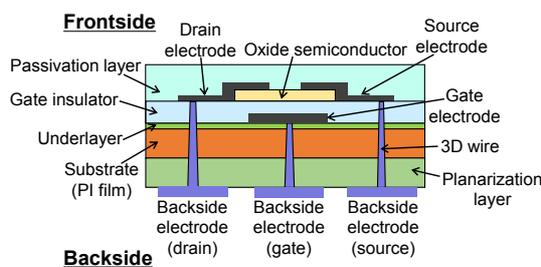
Fig. 1. Cross-sectional view of oxide TFTs driven from substrate backside using 3D wires.
