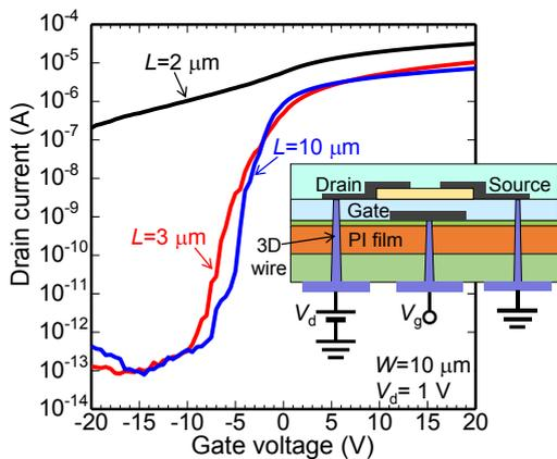
**Fig. 4. Transfer characteristics of BCE-ITZO-TFTs driven from the backside of the PI film substrate using 3D wires.  $V_d$  and  $V_g$  are the drain and gate voltages, respectively.**
