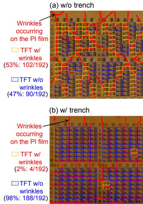
**Fig. 5. Wrinkles on TFT array (192 TFTs) (a) with and (b) without trench structure of  $\text{SiO}_2$  layer after the LLO process.**
