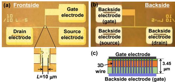
**Fig. 3. Optical micrographs of a fabricated BCE-ITZO-TFT taken from the (a) frontside and (b) backside of the PI film substrate. (c) Cross-sectional view of the structure between the frontside and backside gate electrodes.**
