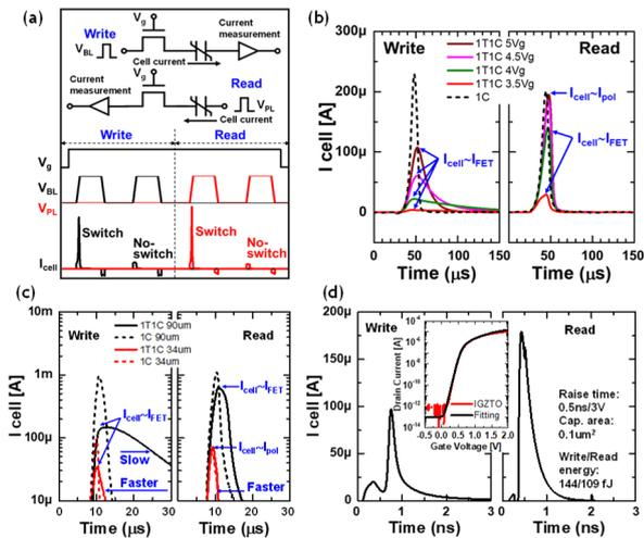
Fig. 11 (a) Measurement setup and typical measured waveform of a 1T1C cell. (b) The measured waveform of the 1T1C cell current with different  $V_g$  and 1C devices. (c) Measured waveform of the 1T1C cell current with different FE-capacitor sizes and 1C device. (d) SPICE simulation with  $0.1\mu\text{m}^2$  capacitor shows ns operation of 1T1C cell. The inset shows FET calibration.
