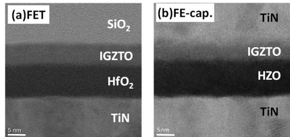
Fig. 5 Cross-sectional STEM images of (a) IGZTO FET and (b) FE-capacitor. Each layer was uniformly formed. With IGZTO capping, the HZO layer was crystallized after RTA.
