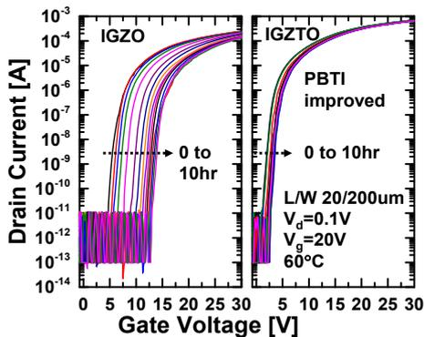
Fig. 3 Measured PBTI characteristics of IGZO and IGZTO FETs made by the baseline process. IGZTO FET shows significant improvement of PBTI reliability.
