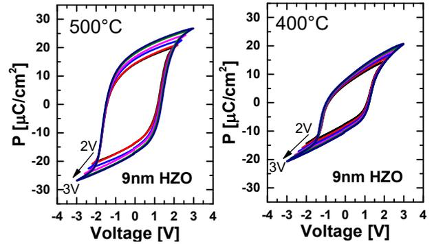
Fig. 9 (Left) Measured P-V curve of an IGZTO-capped HZO FE-capacitor with 500°C RTA. (Right) Measured P-V curve of an IGZTO-capped HZO FE-capacitor with 400°C RTA.
