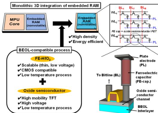
Fig.1 The proposed concept of monolithic 3D integration of oxide semiconductor FET and FE-HfO<sub>2</sub> capacitor for 1T1C embedded RAM application such as eDRAM and FeRAM.
