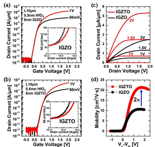
Fig. 6 (a) Measured  $I_d$ - $V_g$  curves of the IGZO FET. The inset shows SS vs  $V_d$ . This is the reference device from Ref. [11]. (b) Measured  $I_d$ - $V_g$  curves of the IGZTO FET. The inset shows SS vs  $V_d$ . Sharp cut-off characteristics are obtained. (c) Measured  $I_d$ - $V_d$  curves of the IGZTO FET and the IGZO FET. IGZTO shows 2 $\times$  higher  $I_{on}$ . (d) Measured effective mobility. IGZTO shows 2 $\times$  higher mobility than IGZO.
