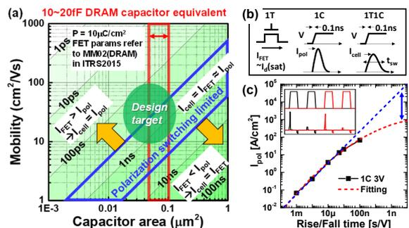
Fig. 2 (a) Contour plot of switching time ( $t_{sw}$ ) of 1T1C cell calculated by FET current ( $I_{FET}$ ) and polarization charge [12]. (b) Definition of  $I_{FET}$ ,  $I_{pol}$ , and  $I_{cell}$ . (c)  $I_{pol}$  with different rise/fall times of voltage pulse.
