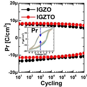
Fig. 10 Measured endurance characteristics without “wake-up” behavior (unstable characteristics in the initial cycles).
