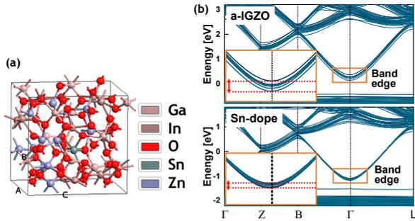
Fig. 8 (a) Atomic structure of an amorphous IGZO. (b) Calculated pseudo-band structures of a-IGZO and IGZTO. 10 samples are shown for each.
