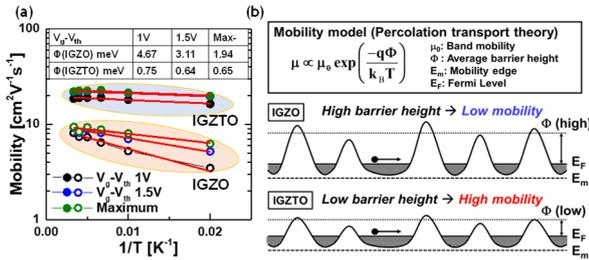
Fig. 7 (a) Temperature dependence of mobility and the extracted average barrier height at different biases. (b) Mobility model based on percolation theory [23]. IGZTO has a lower potential barrier height, which leads to higher mobility.
