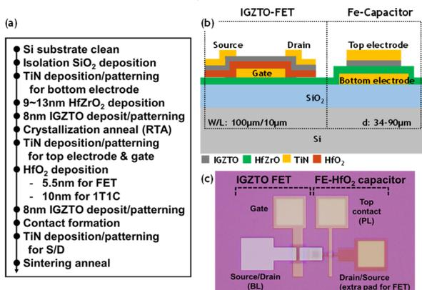
Fig. 4 (a) Fabrication process flow. An IGZTO FET was formed by bottom-gate structure with an ultrathin 8nm IGZTO. A FE-capacitor was formed in the stack of  $\text{TiN}/\text{HZO}/\text{IGZTO}/\text{TiN}$ . (b) Schematic of the device structure. (c) Microscope image. The IGZTO FET and the FE-cap are integrated into the same device.
