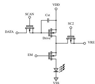
Fig. 2 A Simple Pixel Circuit
