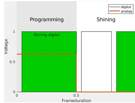
**Fig. 5 Analog vs Subframe Based Digital-driving Scheme**
