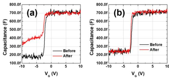
**Fig. 5** (a) Gate to drain and (b) gate to source capacitance as a function of gate bias before and after the doping process
