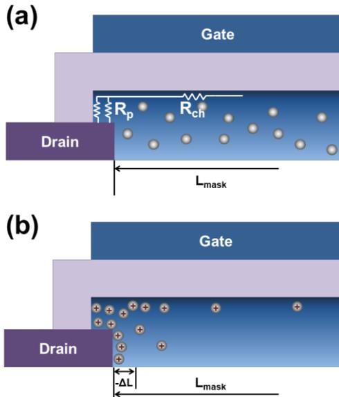
**Fig. 4** Schematic diagrams of resistance elements in a top-gated TFT having bottom contact configuration with (a) un-doped and (b) doped drain region
