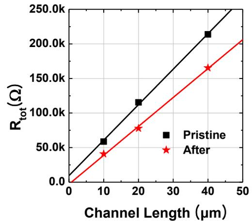
**Fig. 3 Plots of R<sub>tot</sub> as a function of the channel length for pristine state and doped device via proposed method.**
