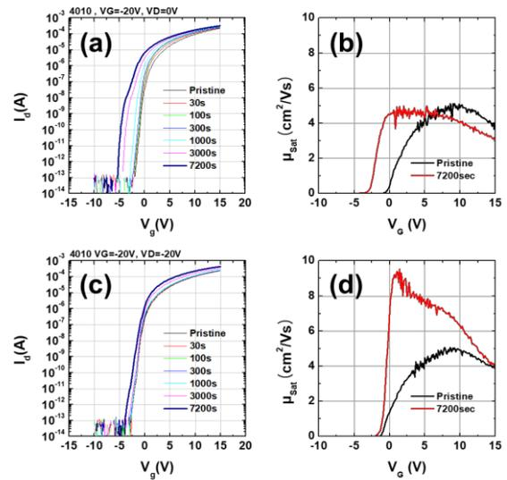
**Fig. 2 Evolutions of transfer characteristics under NBIS condition with drain bias of (a) 0V and (c) -20V as a function of test time. (b) and (d) are the changes in saturation mobility obtained from (a) and (c), respectively.**
