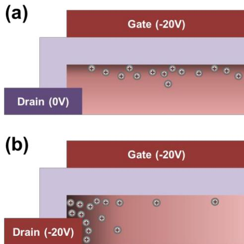
**Fig. 1 Schematics illustrating distribution of positive charges inside a-IGZO under NBIS condition with drain bias of (a) 0V and (b) -20V**
