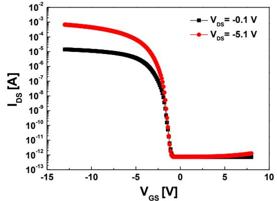
**Fig. 3 I-V transfer characteristics of LTPS TFT.**
