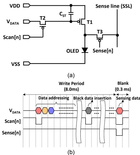
**Fig. 1 Pixel circuit structure (a) circuit schematic (b) timing diagram for 1 frame time (8.3 ms).**
