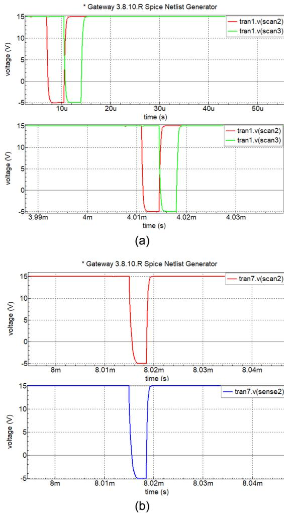
**Fig. 4 Simulation voltage waveforms of (a) Scan[n], Scan[n+1] in write period and (b) Scan[n], Sense[n] in blank period.**
