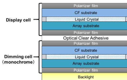
Figure 1. Cross-sectional structure of the dual-cell LCD.
