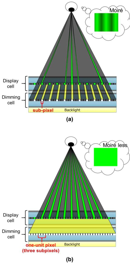
**Figure 4. Monochromatic representation of the developed dual-cell LCD when (a) dimming in each sub-pixel unit or (b) three subpixels as one-unit pixel.**
