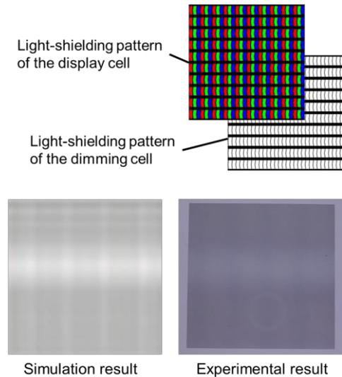
**Figure 3. Comparison of simulation and experimental results for moiré.**
