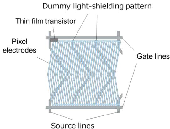
**Figure 8. Improved pixel structures of the dimming cell.**
