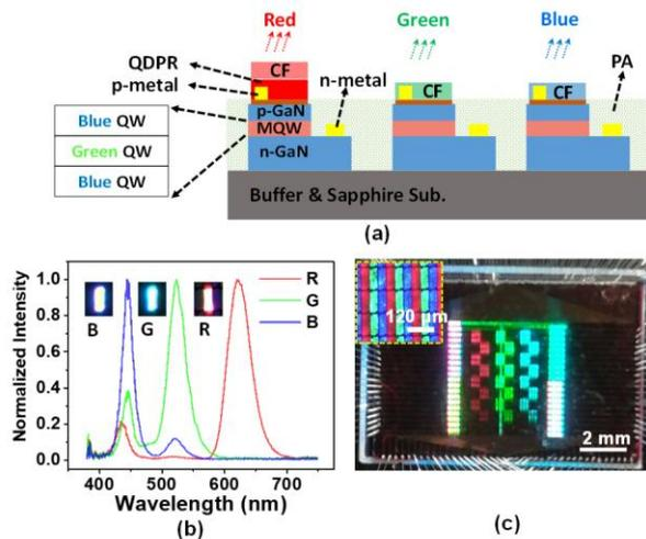
**Fig. 4 (a) Schematic of the full-color micro-display using dual wavelength LED and red QDPR. (b) EL spectra of red, green and blue subpixels. (c) Full-color images rendered on this micro-display.**
