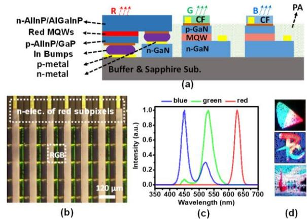
**Fig. 5 (a) Schematic of the full-color micro-display using dual wavelength LED and red AlGaInP micro-LEDs. (b) Image of the display after GaAs substrate removal. (c) EL spectra of red, green and blue subpixels. (d) Full-color images rendered on this micro-display.**
