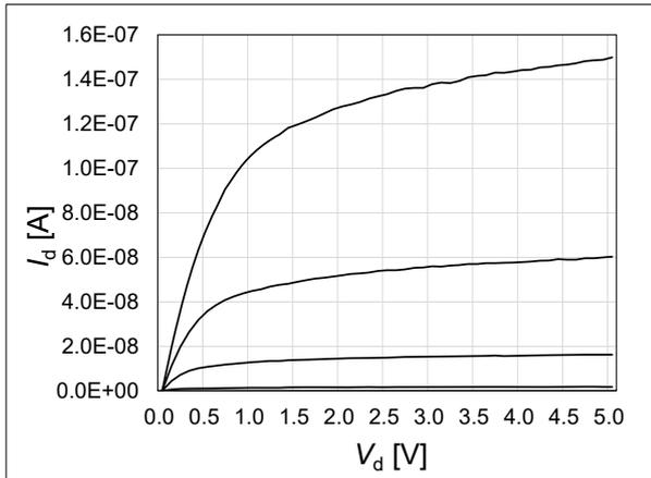
**Fig. 6 Characteristics of OSFET**
