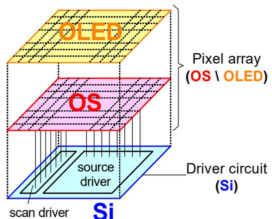
Fig. 1 Conceptual diagram of the Si \ OS \ OLED monolithic stack
