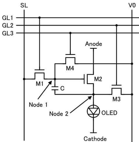
**Fig. 7 Pixel circuit diagram**
