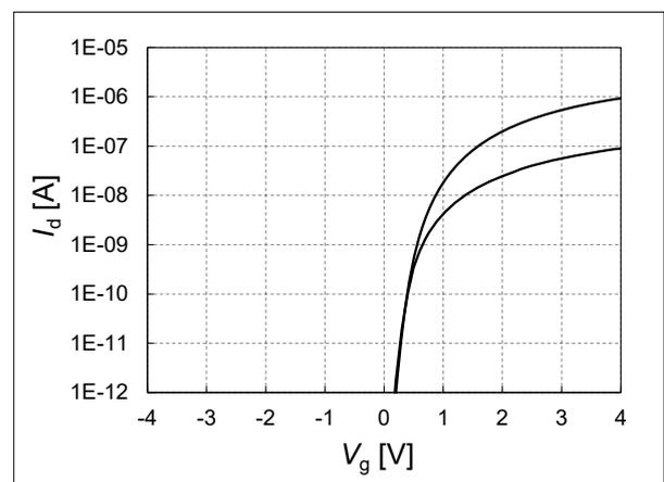
**Fig. 5 Characteristics of OSFET (W/L = 60 nm/200 nm,  $V_{ds} = 0.1$  V, 1.2 V)**
