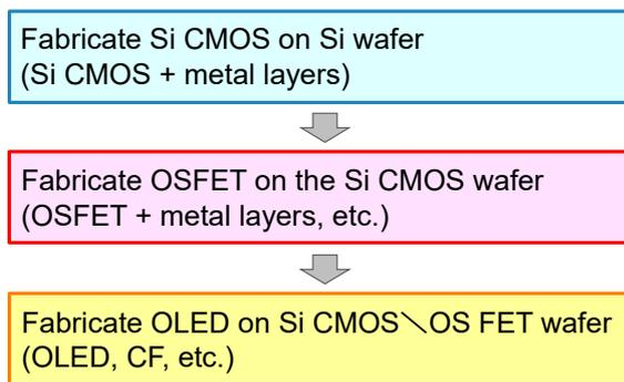
**Fig. 2 Fabrication flow of the Si\OS\OLED monolithic stack**
