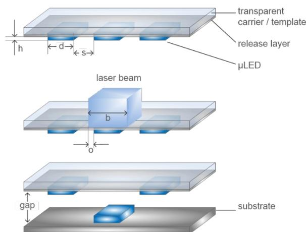
**Fig. 6. Basic conditions for selective MicroLED Mass Transfer**
