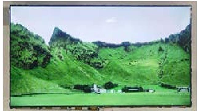
Fig. 6 50 inch UHD 120Hz TFT-LCD panel with the Cu process using 4-mask a-Si TFT
