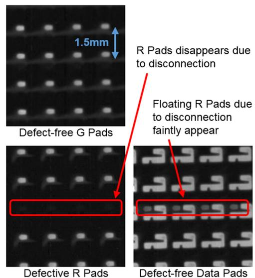
Fig.8 EPIS images of defective Mini-LED substrate
