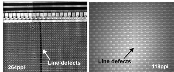
Fig. 4 Capacity inspection of the potential charged in the LCD pixel
