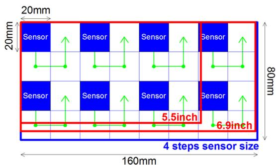
Fig. 9 Sensor tiling arrangement and smartphone panel size
