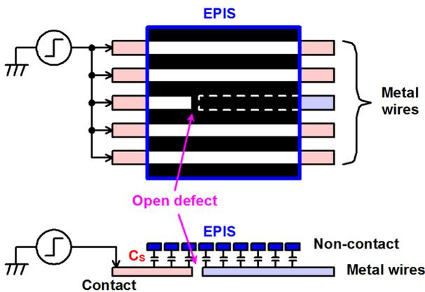
Fig. 2 Flat panel testing method
