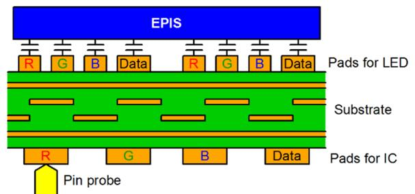
Fig.7 The schematic cross-section of Mini-LED substrate
