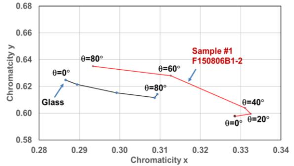
Fig.11 Chromaticity variations of OLEDs with glass and PEN superstrates (S#1) at different measurement angles.
