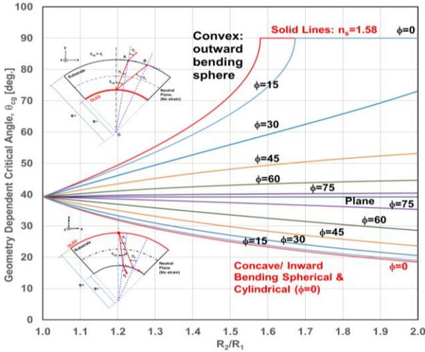
Fig.8 Variation of the geometrical shape dependent critical angle  $\theta_{cg}$  with the inner and the outer radii of the bent superstrate ( $\phi$ : azimuth angle in Fig.5).
