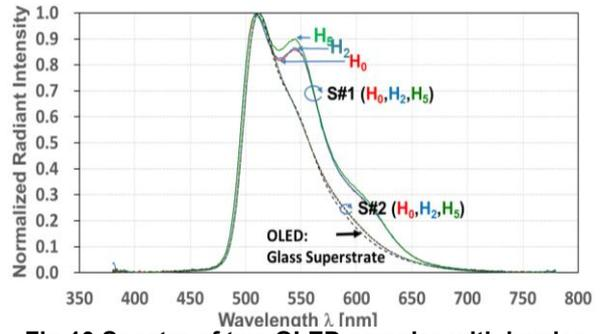
Fig.10 Spectra of two OLED samples with barrier layer of 100 nm and 150 nm, in the planar and the convex states, i.e., the sags of  $H_0=0$  mm,  $H_2=2$  mm,  $H_5=5$  mm.
