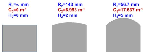
Fig.9 Jigs for bending the OLED samples. The sags of the jigs are  $H_0=0$  mm,  $H_2=2$  mm, and  $H_5=5$  mm.
