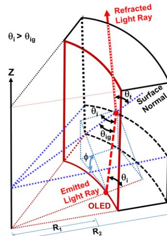
Fig.5 Geometry of the convex cylindrical OLED.
