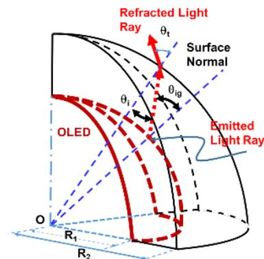
Fig.4 Geometry of the convex spherical OLED.
