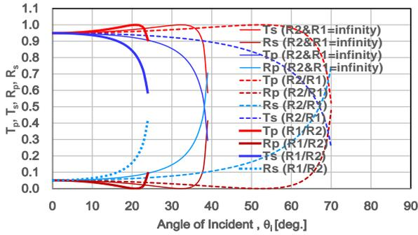
Fig.6 Transmission (upper,  $T_s, T_p$ ) & reflection (lower,  $R_s, R_p$ ) coefficients in the planar, the concave and the convex spherically bent OLED superstrate with inner and outer radii of  $R_1$  and  $R_2$ .
