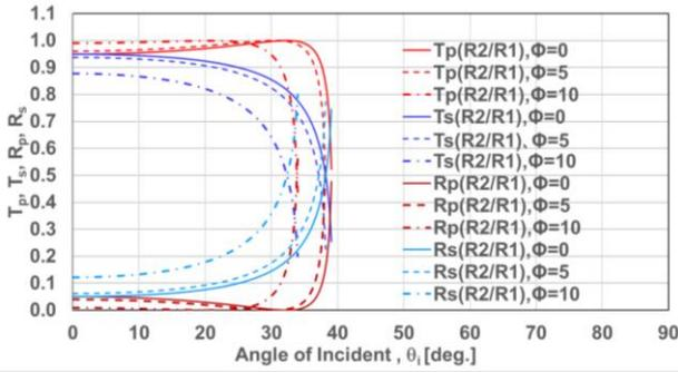
Fig.7 Reflection and transmission coefficients in the convex spherical ( $\Phi=0$ ), and the cylindrical convex ( $\Phi>0$ ) OLEDs with inner and outer radii of  $R_1$  and  $R_2$ .
