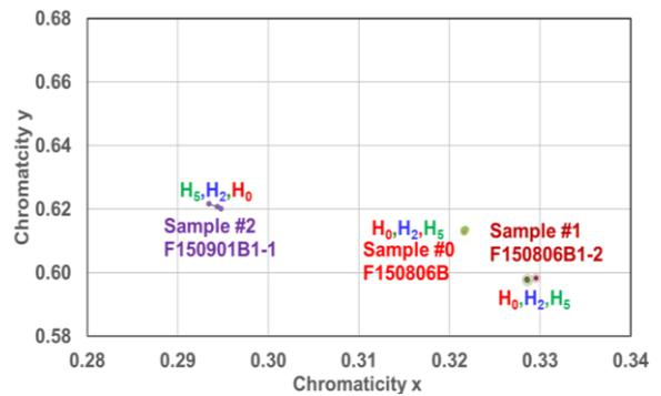
Fig.12 Chromaticity variations of OLEDs with PEN superstrates at the cylindrically curved states (on surface normal direction). S#0: for comparison.
