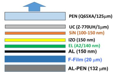
Fig.1 Structure of the fabricated OLED (Top emission)
