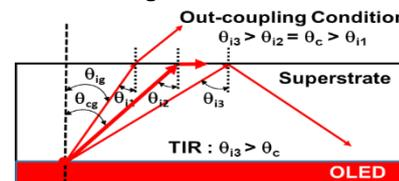
Fig.3 A planar OLED and the refraction/reflection of the emitted light in the superstrate.
