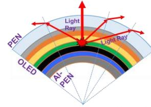
Fig.2 Schematic diagram of the OLED in bent state.
