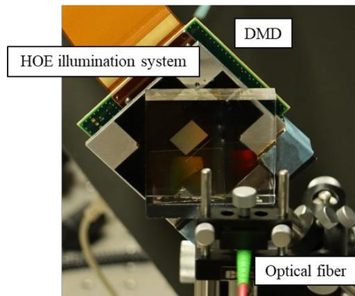
**Fig. 5 Display system using pulse-modulated MEMS SLM with HOE illumination system.**
