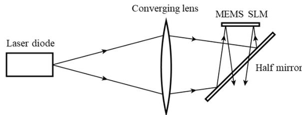
**Fig. 2 Illumination system used for previous display system using pulse-modulated MEMS SLM.**
