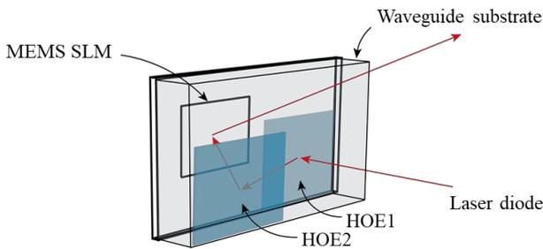
**Fig. 3 Proposed pulse-modulated MEMS SLM with HOE illumination system.**
