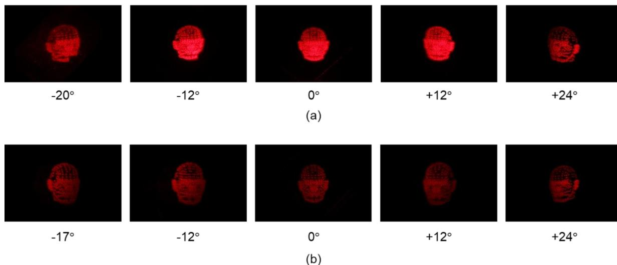
**Fig. 6 Reconstructed images obtained using (a) HOE illumination system, and (b) previous illumination system using half mirror.**
