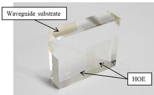
**Fig. 4 Fabricated HOE illumination system.**
