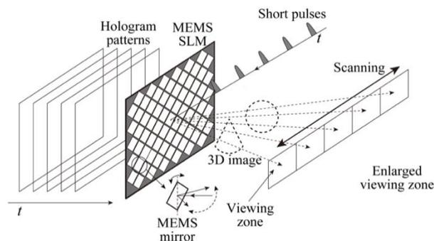
**Fig. 1 Holographic display system using pulse-modulated MEMS SLM.**
