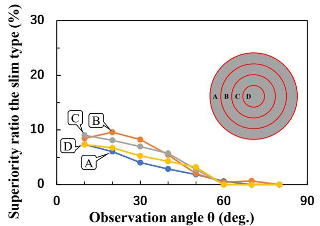
Figure 11. Superiority of visible display volume at the slim type screen compared with the fat type in the 4 donut areas
