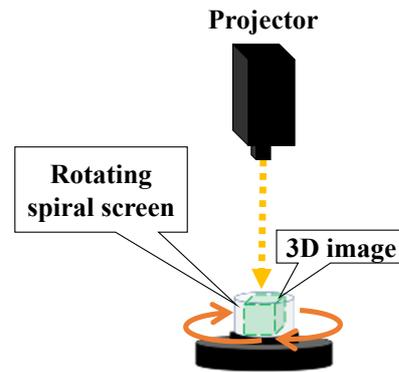
Figure 1. Arrangement of the proposed 3D display system
