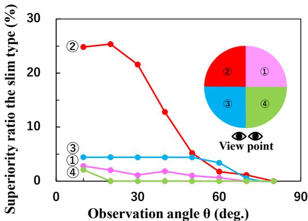
Figure 8. Superiority of visible display volume at the slim type screen compared with the fat type in each quadrant
