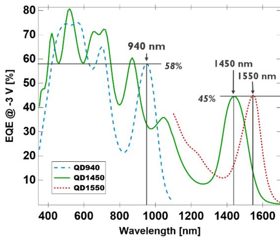
Fig. 3 External quantum efficiency of 6.25 mm<sup>2</sup> photodiodes on silicon (top illuminated)
