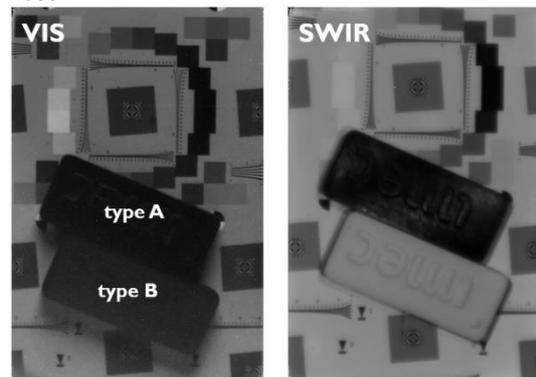
Fig. 5 Scene acquired with the same QD image sensor in the visible (left) and SWIR range (right). The latter is taken through a Si wafer.
