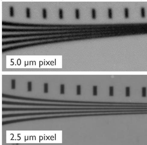
**Fig. 6 Images acquired with QD image sensors with the pixel pitch of 5  $\mu\text{m}$  (top) and 2.5  $\mu\text{m}$  (bottom)**
