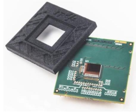
Fig. 4 Packaged QD image sensor
