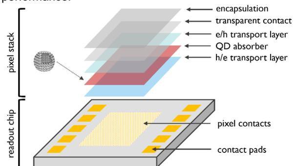
Fig. 2 Pixel stack based on quantum dot absorber
