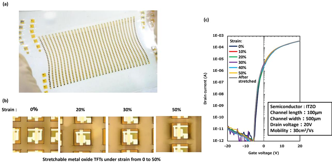
**Fig. 5. (a) photograph of the stretchable metal oxide TFT under 50% strain. (b) Photograph of a stretchable metal oxide TFT on an elastomer with acrylic adhesive. (c) Transfer characteristics of the metal oxide transistor stretched by 0%, 10%, 20%, 30%, 40%, 50%, and released to 0%.**
