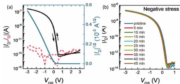
**Figure 2. Transfer characteristics and bias-stress stability of an all-inkjet-printed OTFT [7].**
