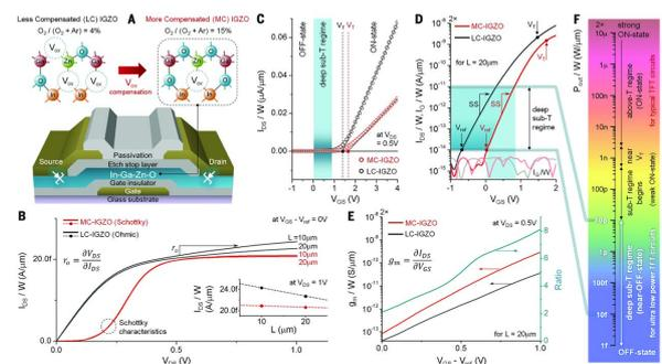
**Figure 4. Device structure and basic electrical characteristics of a Schottky-barrier TFT realized using vacuum-deposited semiconductor oxide technology [8]**
