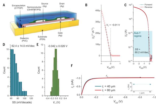
**Figure 3. Schematic cross section and electrical characteristics of the fabricated OTFT [5].**
