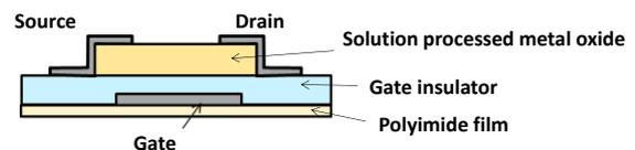
**Fig. 3. Photograph of the direct patterned metal oxide TFT on plastic substrate and a schematic diagram of fabricated TFT structure.**
