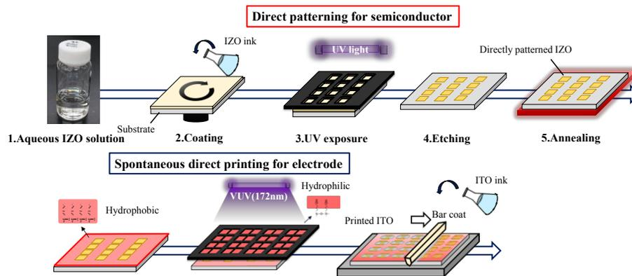
**Fig. 4. Process flow for printed metal oxide TFTs using a direct patterning for semiconductor and spontaneous direct printing process for ITO inks.**
