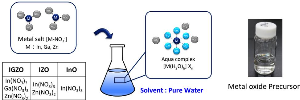
**Fig. 2. Carbon-free aqueous metal oxide precursor for low-temperature processing. Aqueous IGZO, IZO, and InO precursor are synthesized by only nitrate salts and pure water.**
