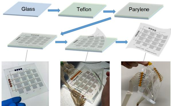
**Fig. 2 Fabrication process of ultra-flexible proximity sensor array. Reproduced from [5] with permission of John Wiley & Sons.**
