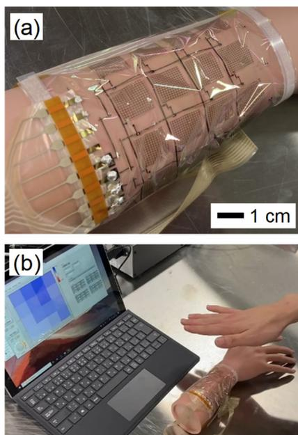
**Fig. 5 Proximity sensing with ultra-flexible array. Reproduced from [5] with permission of John Wiley & Sons.**
