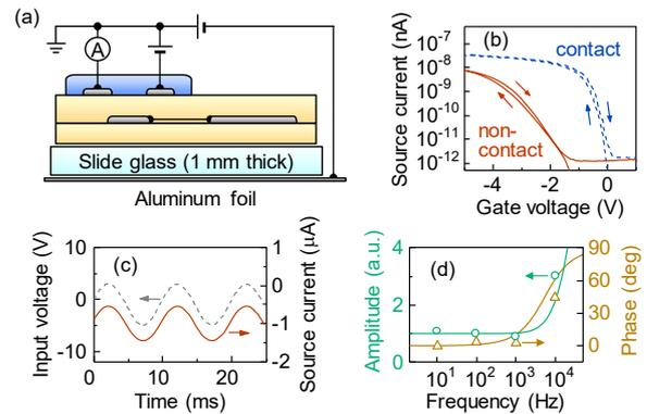
**Fig. 3 Device characteristics. (a) Non-contact mode. (b) Transfer characteristics in contact and non-contact modes. (c) Response to sinusoidal input at 100 Hz. (d) Frequency characteristics. Reproduced from [5] with permission of John Wiley & Sons.**
