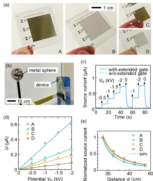
**Fig. 4 (a) Photographs of FEG-OFETs. (b) Experimental setup. (c)(d) Dependence of current on potential at  $d = 15 \text{ cm}$ , and (e) on distance at  $V_0 = -2 \text{ kV}$ . Reproduced from [5] with permission of John Wiley & Sons.**
