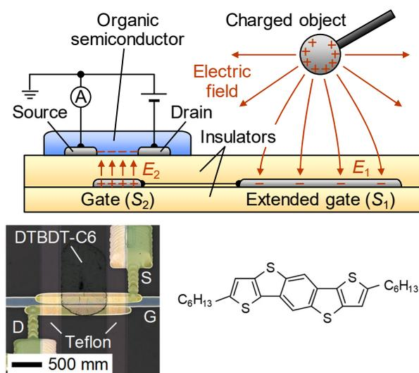
Fig. 1 (a) Schematic and (b) optical microscope image of floating extended gate organic field-effect transistors (FEG-OFET). (c) Structure of DTBDT-C6. Reproduced from [5] with permission of John Wiley & Sons.
