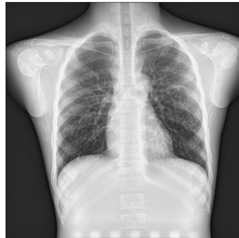
Fig. 8 Example of chest phantom image obtained using the ISS system flexible FPD with the CsI scintillator.
