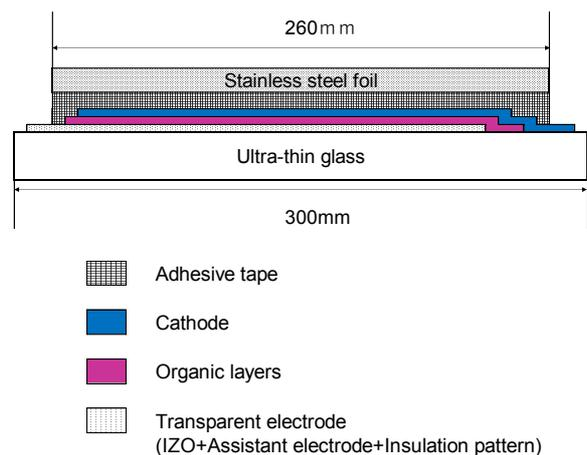
Fig. 1 Device structure
