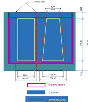
Fig. 6 Position of the deposited organic and metallic cathode layers
