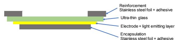
Fig. 17. Reinforcement for the device
