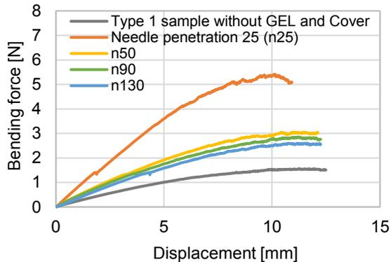
**Fig. 5** The relationship between the bending force and the pressing displacement depending on the hardness / modulus of the OPTαGEL.
