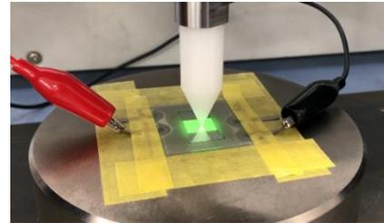
Fig. 3 Pressing rod on the OLED lighting.
