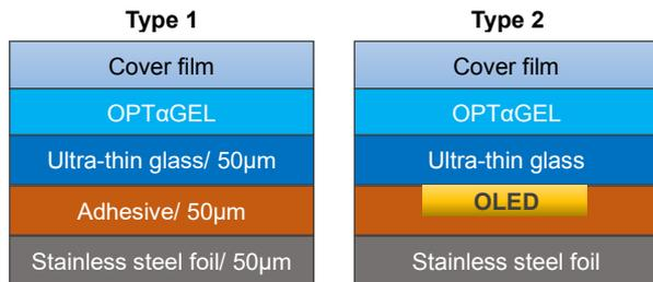
Fig. 1 Test sample configuration.
