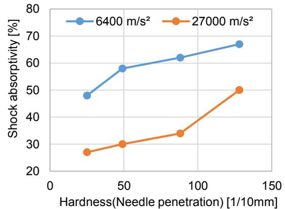
**Fig. 7** Shock absorptivity depending on hardness of OPTαGEL.
