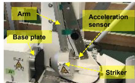
Fig. 4 Pendulum shock absorptivity testing equipment.
