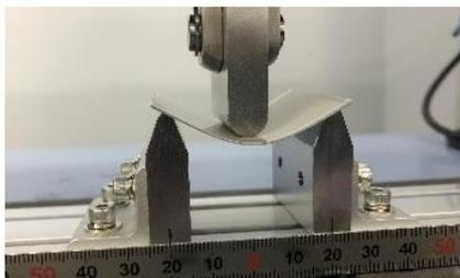
Fig. 2 Bending test jig and a test sample.
