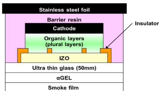
**Fig. 8 The structure of the OLED lighting.**
