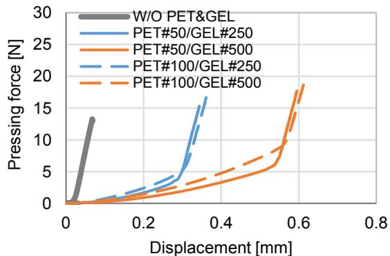
**Fig. 6** The relationship between the pressing force and the displacement of the OLED lightning device with the protection layer.
