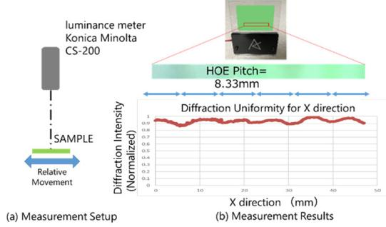
Fig. 5 Diffraction Uniformity Measurement
