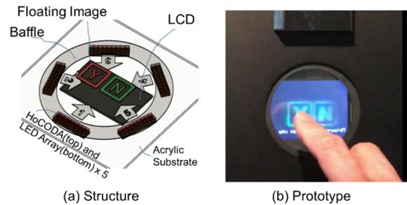
Fig. 7 Contactless Input UI
