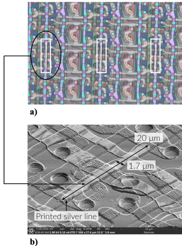
Figure 3 a) Repeatable and continuous silver lines with a width of 1.7  $\mu\text{m}$  and length of 20  $\mu\text{m}$  printed on OLED substrate. b) Magnification of the selected line.
