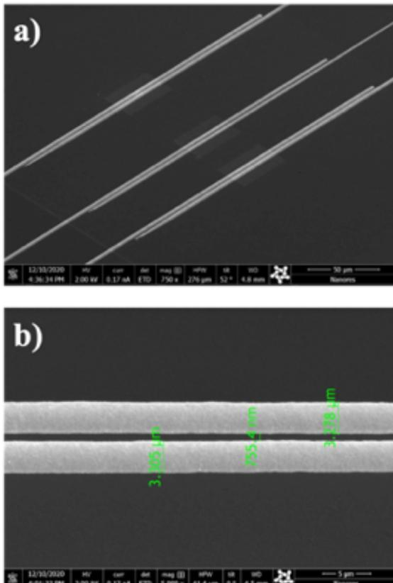
Figure 2 a) Example set of silver lines printed on a PEN foil, b) magnification of the sample.
