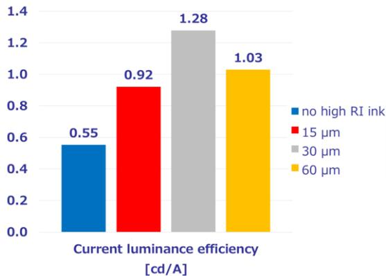
**Fig. 5. Current luminance efficiency when changing film thickness of HRI material.**
