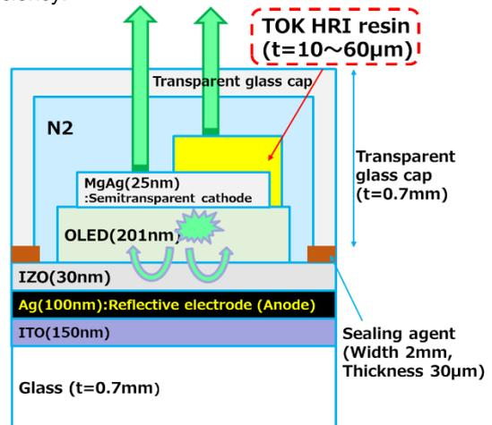
Fig. 2. OLED device structure.
