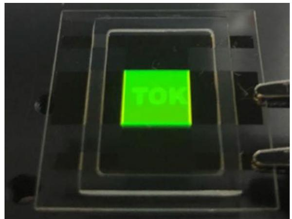
**Fig. 4. Emission of the OLED device in which the characters TOK are printed by HRI ink.**
