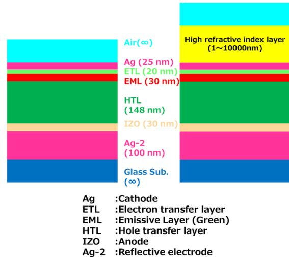
Fig. 1. OLED device models without HRI layer (left) and with HRI layer (right) for the simulation.
