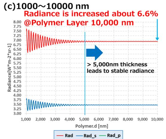
**Fig. 3. Simulated radiance of (a) 1~100 nm; (b) 100~1000 nm, (c) 1000~10000 nm thickness of HRI ink layer. (Red line is total radiation. Blue and green line indicate radiation of s-polarized and p-polarized light respectively.)**
