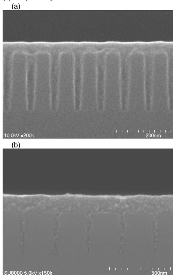
**Fig. 6. SEM image about gapfill.**
