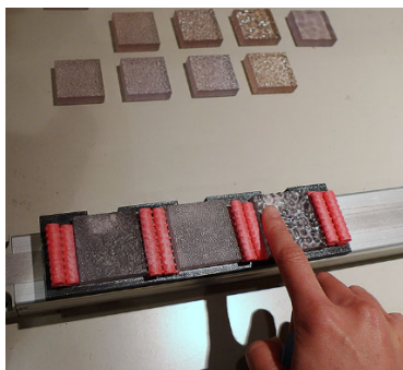
Fig. 4 Experimental setup. The linear stage moved from left to right. The start and end of the stage movement always occurred when the finger was on the cushions (pink in the figure).
