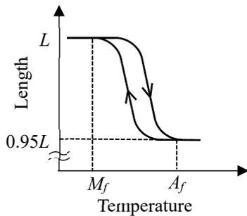
**Fig. 2 Temperature characteristics of SMA**
