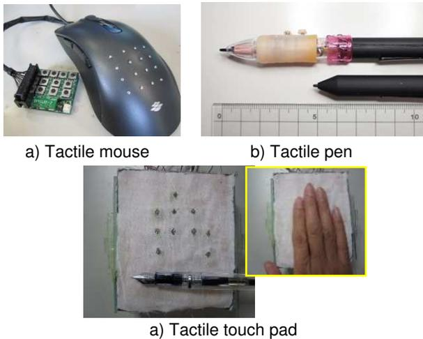
Fig. 6 Examples of Tactile displays
