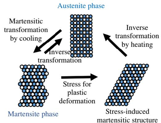
**Fig. 1 Shape memory effect of SMA**
