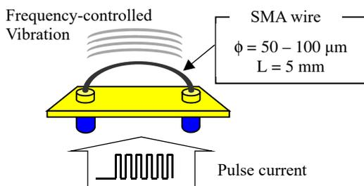
**Fig. 4 Micro-vibration actuator using SMA wire**
