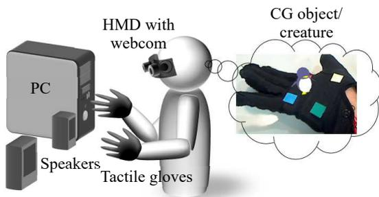
**Fig. 8 AR interaction system with tactile gloves**
