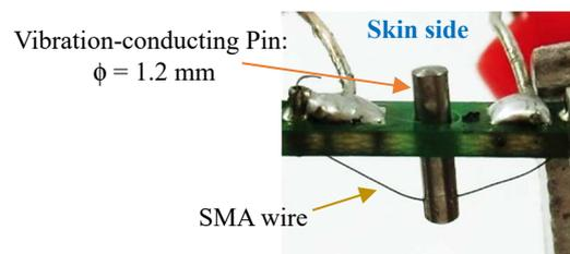
**Fig. 5 Pin-type vibration actuator**
