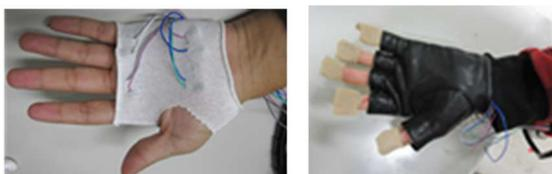
**Fig. 9 Tactile glove with 19 SMA actuators inside**
