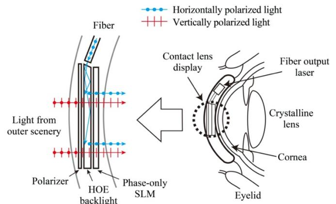
**Fig. 2 Structure of holographic contact lens display**
