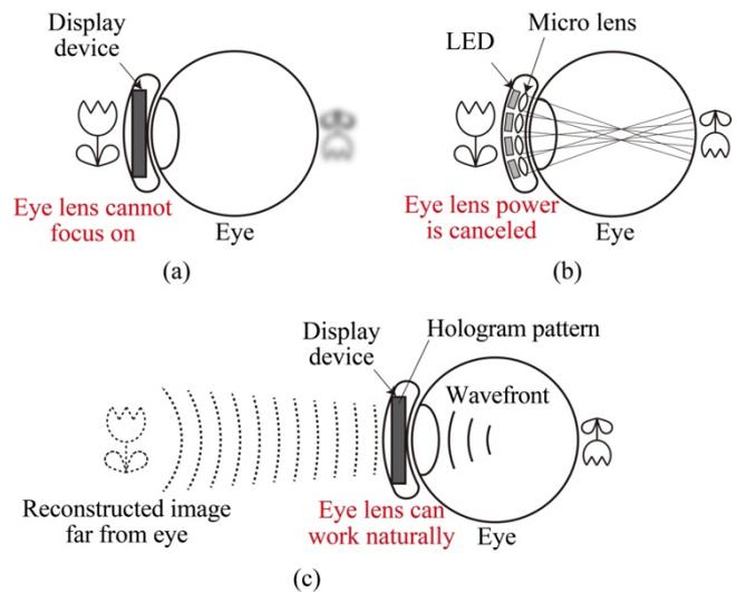
**Fig. 1 Concept of holographic contact lens display: (a) problem, (b) conventional solution, and (c) proposed technique**
