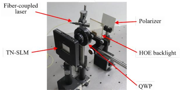
Fig. 3 Constructed bench-top experimental system
