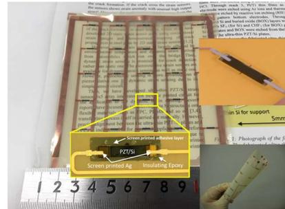
Figure 1. 5x5 ultra-thin PZT/Si strain sensor array for structural health monitoring [6].
